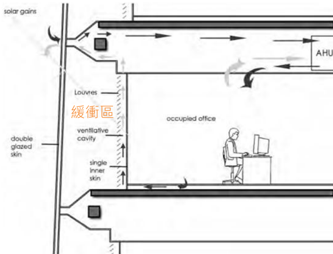
Figure 20.22 Cooling strategy (summer) for Swiss Re Tower
